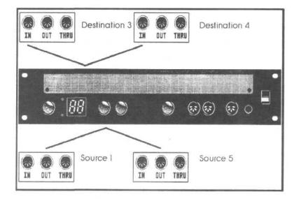
depress the [Up] key until the second digit of the display reads an <M> (which stands for "Merge").
