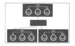
Now, if you want to have one MIDI device controlled by two instruments simultaneously, you need a device that is able to mix two MIDI signal packages. A simple two-way adapter, as is often used for audio connections, cannot be used here because MIDI signals are digital signals and for merging them a special processor is required.
