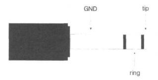
The respective function will be activated by connecting the corresponding contact to GND.
