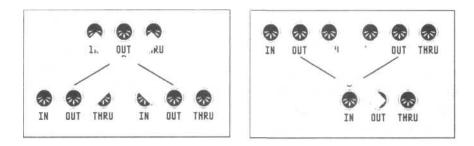
The MIDI specification determines that one MIDI OUT is assigned to each MIDI IN. However, if you want to transmit one MIDI signal to several instruments, there are exactly two ways to do so:
